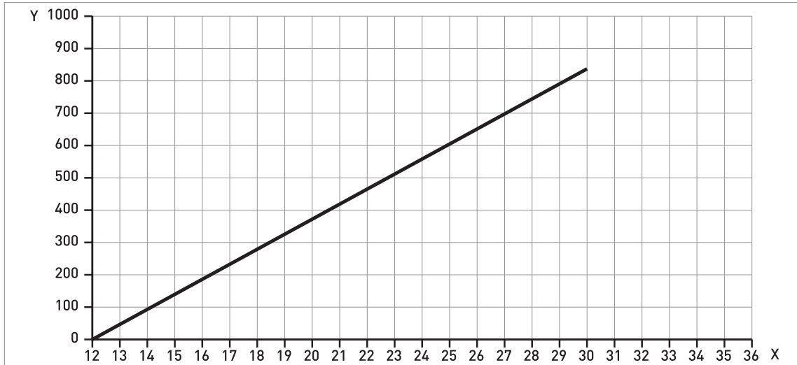
Figure 2-1: Minimum power supply voltage for an output of 21.5 mA at the terminals (Non-Ex and Hazardous Location approval (Ex i / IS))
