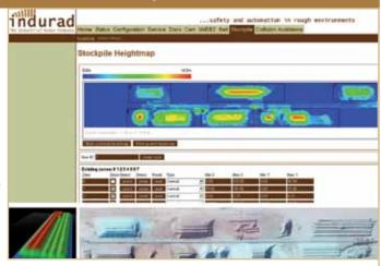
The indurad iWEB™ is a human machine interface (HMI). Access is as easy as opening a webpage. iWEB™ allows secured access to all required information for setup, parameterization as well as visualization and process analysis. Cost intensive SCADA integration is avoided, no software installation is required.
