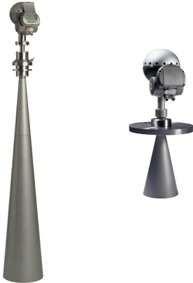
Pro Hot has a shorter cone antenna with purging, the Pro's standard wave-guide connection and digital signal processing using FFT and the software modules Echofixer and optional FHAST. It is less superior than Pro Steel during charging and has a shorter measuring range but is the answer for "low cost" but still reliable measurement suitable for normal operation. Pro Hot is the best alternative compared to other "cheap" gauges. For more information see the specifications on next page.
