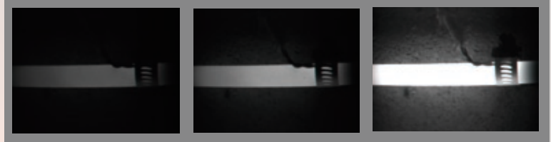
Actual VIS THERMALVISION™ Camera measuring rod temperatures 750°F [400°C] - 2865°F [1575°C]
