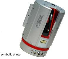
Detailed specifications and laser classification according to the latest datasheet *RIEGL* VQ-180.
