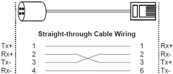
**Attention:** use OVP (overvoltage protection devices) for longer Ethernet cable lengths and/or outdoor use, the max. allowed cable length of 100 m (refer to TIA-EIA-568-B.2) applies to the total length of the cable between two active devices / incl. both sides of the OVP!
